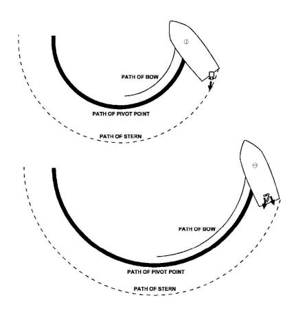
Figure 6-19 Pivot Point, Skid, Kick, Inboard vs. Outboard
