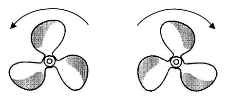
VIEWED FROM ASTERN, TURNING FOR PROPULSION TO GO AHEAD. PROPELLER ON RIGHT (STARBOARD SHAFT) TURNS CLOCKWISE AND IS CALLED A RIGHT-HANDED PROPELLER. WHEN BACKING, ROTATION IS OPPOSITE.
