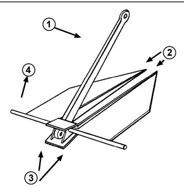
Figure 6-32 Main Parts of a Danforth Anchor
