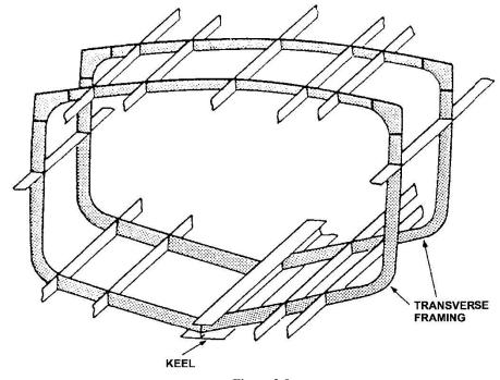
Figure 3-9 Transverse Framing System
