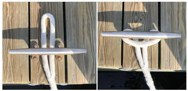
Figure 2-37 Securing a Dock Line to a Cleat
