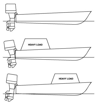
Figure 6-11 Trim to Offset Loading Condition
