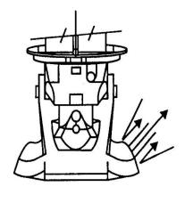
To move the vessel's stern to port, the tiller is moved to starboard to direct thrust away from the boat off its starboard quarter. The throttle/bucket control is centered to perform a stationary pivot or may be moved aft to increase the speed of the maneuver.
