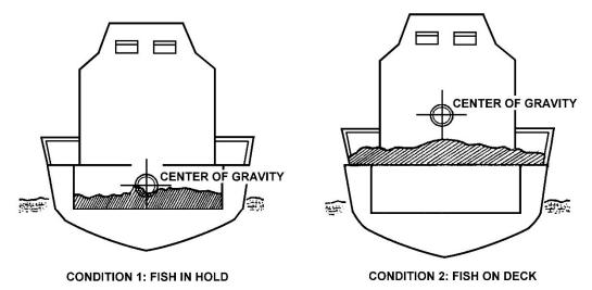
Figure 4-5 Effects of Load Weight
