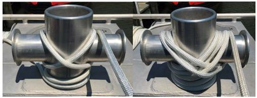
Figure 2-35 Securing a Line to a Single Bitt
