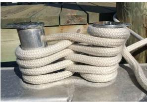
Figure 2-34 Securing a Line to Paired Bitt
