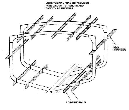
Figure 3-10 Longitudinal Framing System
