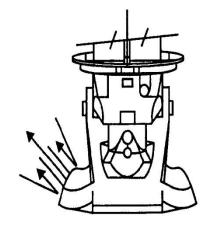
To move the vessel's stern to starboard the helm is turned to port and the bucket control is moved aft to direct thrust away from the boat off its port quarter. The throttle is lowered to perform a stationary pivot or may be moved to increase the speed of the maneuver.
