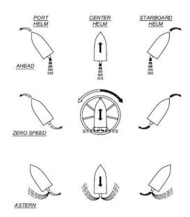
Figure 6-15 **Thrust and Directional Control**
