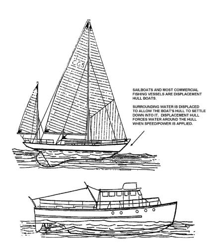
Figure 3-3 Displacement Hulls
