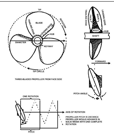
Figure 3-8 Parts of a Propeller
