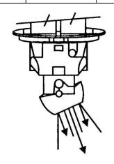
To turn the bow to starboard the helm is turned to starboard and the bucket control is moved forward to direct thrust away from the boat off its starboard quarter. The throttle is lowered to perform a stationary pivot or may be forward to turn at speed.
