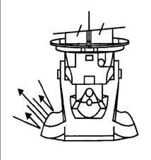
To move the vessel's stern to starboard, the tiller is moved to port to direct thrust away from the boat off its port quarter. The throttle/bucket control is centered to perform a stationary pivot or may be moved aft to increase the speed of the maneuver.
