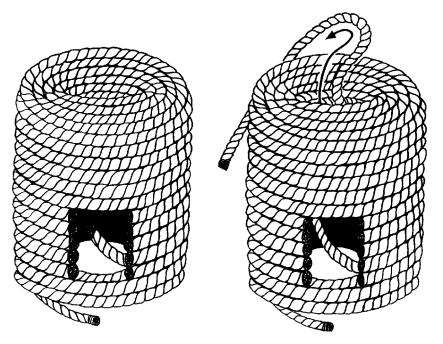
Figure 2-3 Opening a New Coil of Line
