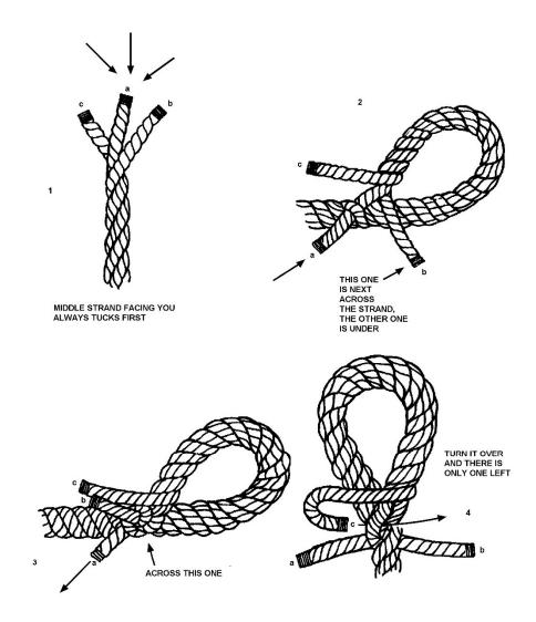
Figure 2-25 Three-Stranded Eye Splice
