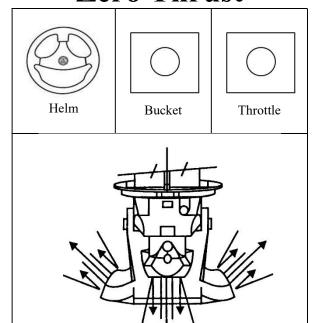
Zero thrust is achieved by centering the helm and throttle controls and by moving the bucket control to a point where thrust is directed so the boat maintains position.
