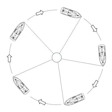
Figure 6-36 Freeing a Fouled Anchor
