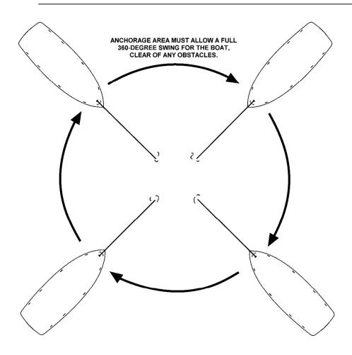
Figure 6-34 **Anchorage Swing Area**
