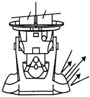
To move the vessel's stern to port the helm is turned to starboard and the bucket control is moved aft to direct thrust away from the boat off its starboard quarter. The throttle is lowered to perform a stationary pivot or may be moved to increase the speed of the maneuver.
