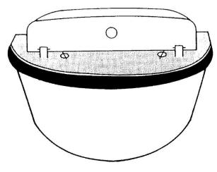
Figure 3-5 Rounded, Cruiser-Type Stern
