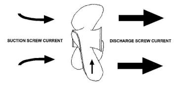
PROPELLER IS VIEWED FROM PORT SIDE WITH NEAREST BLADE ROTATING UPWARD (RIGHT-HANDED)
