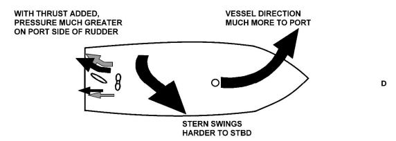
Figure 6-8 Effect of Rudder Action
