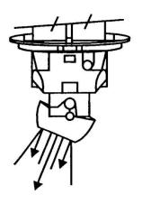
To turn the bow to port the helm is turned to port and the bucket control is moved forward to direct thrust away from the boat off its port quarter. The throttle is lowered to perform a stationary pivot or may be forward to turn at speed.
