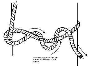
Figure 2-16 Timber Hitch
