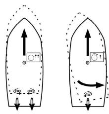
TWIN-SCREW VESSEL ACCELERATES IN A STRAIGHT LINE. SINGLE-SCREW VESSEL IS AFFECTED BY SIDE FORCE, STERN "WALKS" TO STARBOARD. OFFSET FOR SIDE FORCE WITH SLIGHT RIGHT RUDDER.
