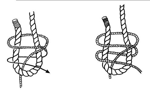
Figure 2-19 Double Becket Bend/Sheet Bend
