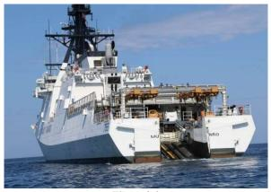
Figure 3-2 Tumble Home Hull Design
