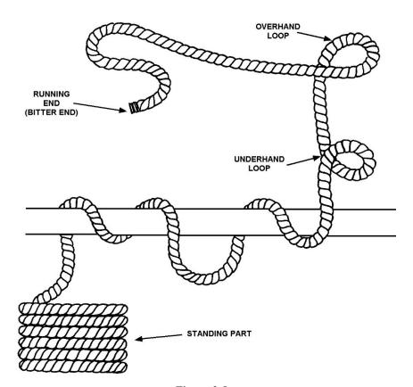
Figure 2-8 Basic Parts and Loops
